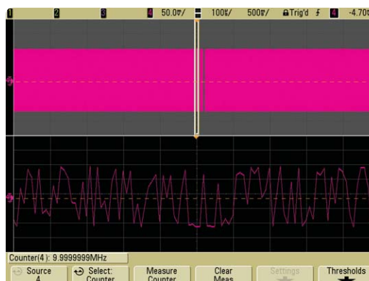
Figure 13. Built-in hardware counter allows for making 8-digit frequency measurement using an external 10 MHz reference input.
