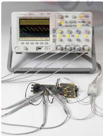
Figure 2. The 4+16-channel MSO allows you to view up to 4 analog and 16 digital signals on one instrument.
